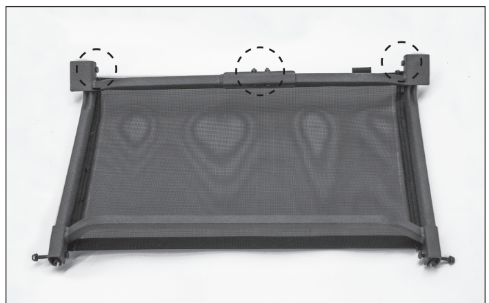
FIGURE 14 - Tighten the four front brace bolts and locknuts
