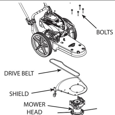
**FIGURE 20:** Mower Head Housing and Shield
