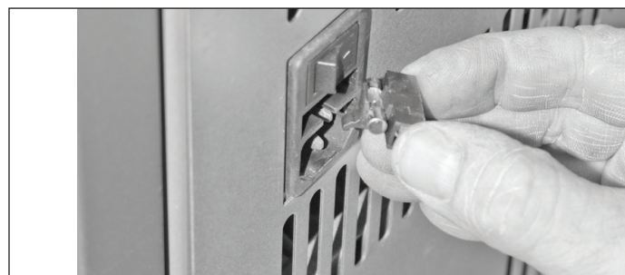
Figure 20b: Main power switch
