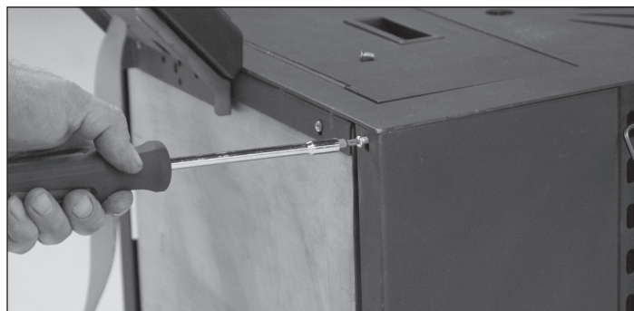
Figure 35: Remove (2) screws from rear of side panel, at the top and bottom of the panel. Remove (2) screws from the front face of the side panel, at the top and bottom of the panel.
