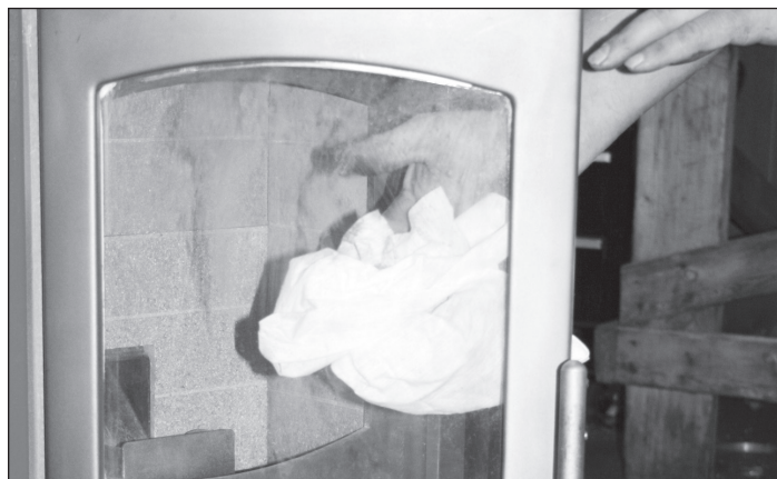
Figure 31: Wipe glass and inspect gasket
