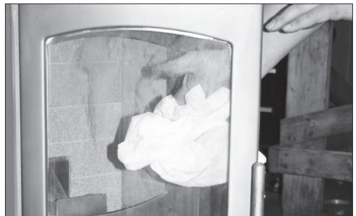
Figure 31: Wipe glass and inspect gasket
