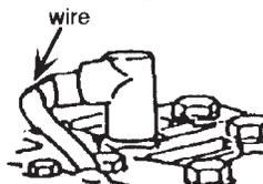
Engine must be turned off and cool, and spark plug wire must be removed and secured from spark plug before checking and adjusting engine or equipment.
