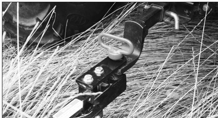
Figure 31: Pin style hitch illustration. NOTE: Use a hitch pin designed to be used with your ATV or garden tractor.
