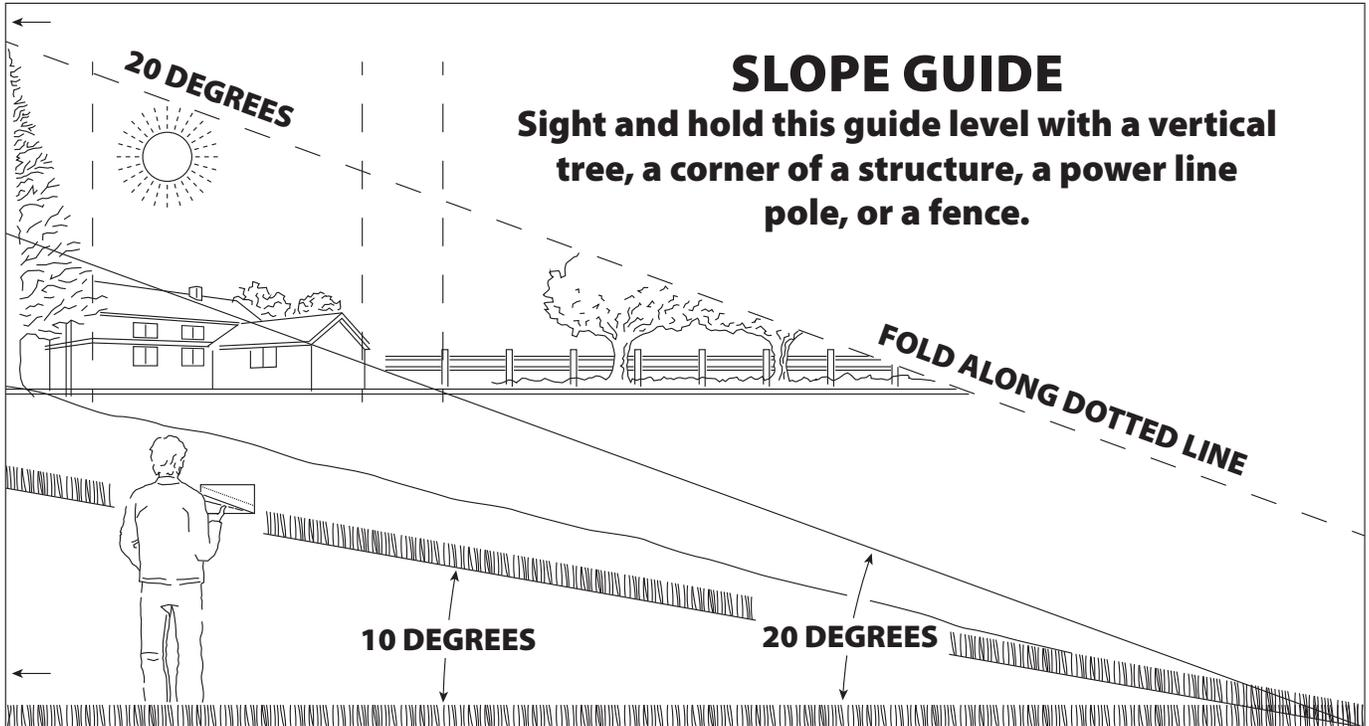
Use this guide to determine slope angle.
