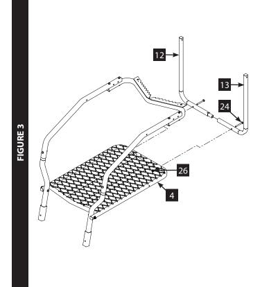
4. Attach right (12) and left (13) rear seat supports to platform (4) using two 1/4-20 X 2-1/4 IN bolts (24) and locknuts (26). **SEE FIGURE 3.**
