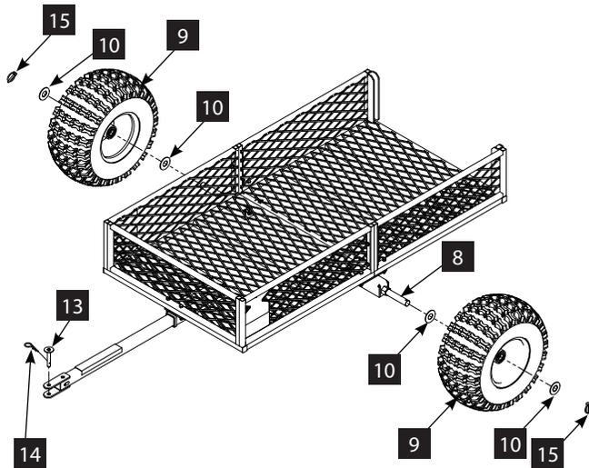
5. Tighten all nut and bolt assemblies. Be sure not to over tighten or crush tubing when tightening.
