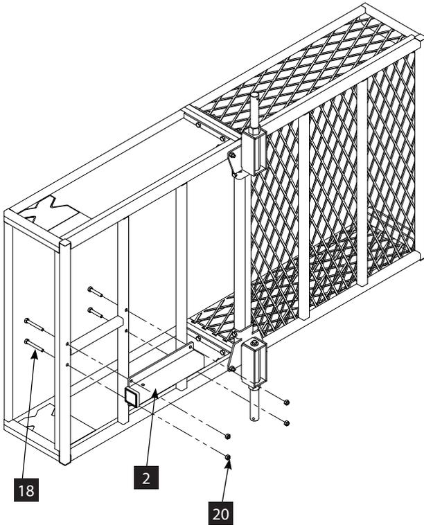
3. Attach the tongue receiver (2) to the front trailer frame (5) using two 5/16-18 x 2 1/2 IN bolts (18), two 5/16-18 x 1 3/4 IN bolts (17), and four nuts (20).
