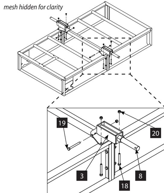
2. Attach each spindle bracket (3) to the bottom of the trailer frames (5 & 6) using two 5/16-18 x 2 ½ IN bolts (18), one 5/16-18 x 3 IN bolt (19), and three nuts (20).
