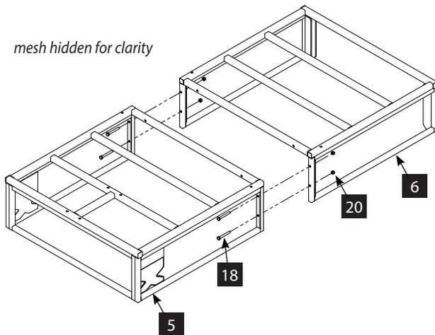
1. Attach front and rear trailer frames (5 & 6) using four 5/16-18 x 2 ½ IN bolts (18) and nuts (20).
