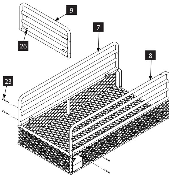
1. Fold side rail left and right (7 & 8) up and attach front rail (9) to both side rails using four 5/16-18 x 2-1/2 IN bolts and nuts (23 & 26).
