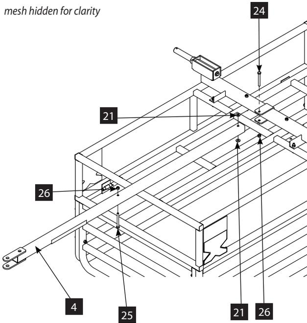
4. Attach trailer tongue to axle using one 5/16 x 18 x 2-3/4 IN bolt, two 8.1 x 19 x 3.5 MM plastic spacers, and one nut (24, 21, & 26). Attach trailer tongue to trailer bed using one 5/16-18 x 3-1/4 IN bolt and nut (25 & 26).
