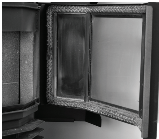
Figure 15: Wipe glass and inspect gasket
