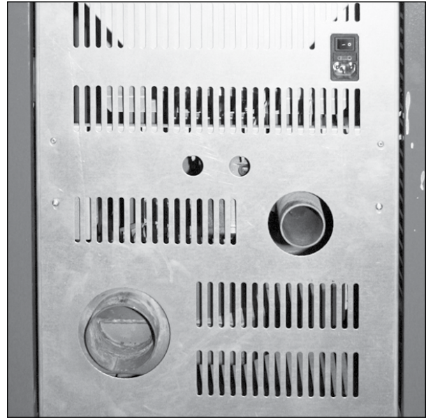
Figure 7: Intake and exhaust positions
