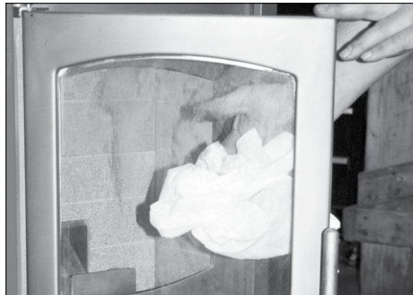
Figure 15: Wipe glass and inspect gasket
