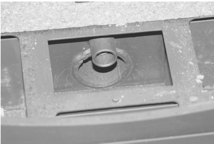
Figure 35: Remove ash from ignitor tube (underneath firepot)
