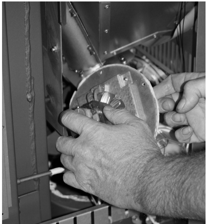
Figure 37: Remove combustion motor and clean
