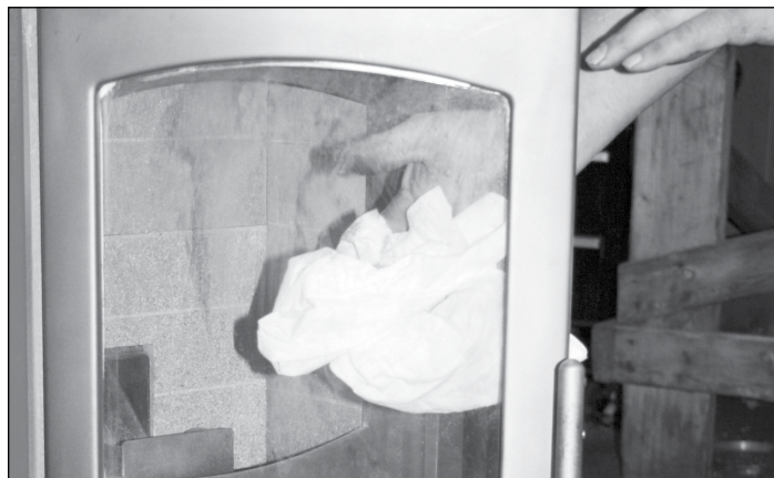
Figure 31: Wipe glass and inspect gasket
