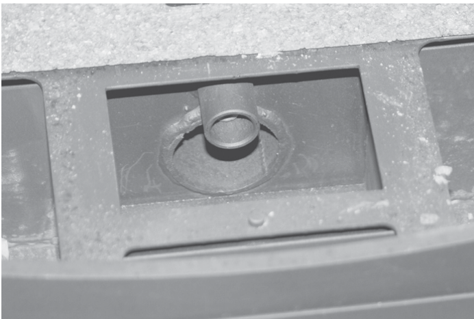
Figure 35: Remove ash from ignitor tube (underneath firepot)
