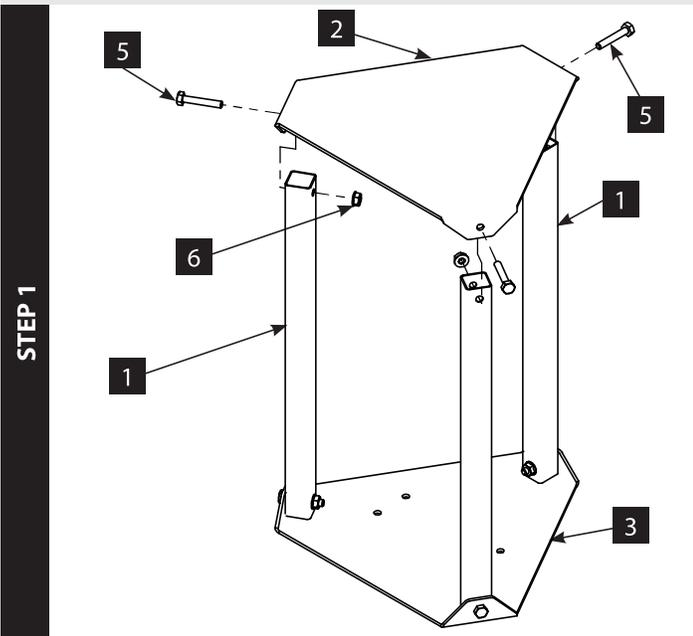
1. Attach the three seat supports (1) to the seat plate (2) and base plate (3) using six 1/4 X 1-1/2 IN bolts (5) and nuts (6). **SEE FIGURE 1.**
