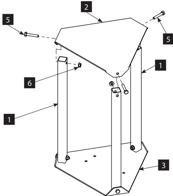
1. Attach the three seat supports (1) to the seat plate (2) and base plate (3) using six 1/4-20 X 1-1/2 IN bolts (5) and 1/4-20 nuts (6). **SEE FIGURE 1.**
