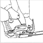
8. When firing occurs, push in the choke knob and pull the starter again to start the engine.
