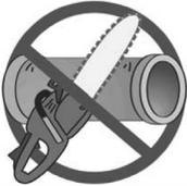
Always follow the safety regulations. The chain saw must only be used for cutting wood. It is forbidden to cut other types of material. Vibrations and kickback vary with different materials and the requirements of the safety regulations would not be respected. Do not use the chain saw as a lever for lifting, moving or splitting objects. Do not lock it over fixed stands. **DO NOT** hitch tools or applications to the P.T.O. that are not specified by the manufacturer.
